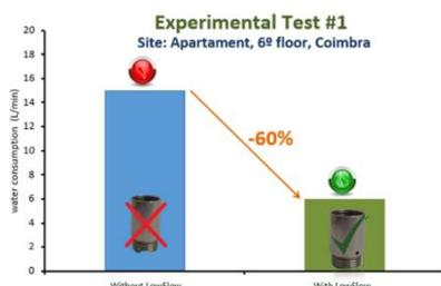
Fig. 7. Water Savings at an apartment.
