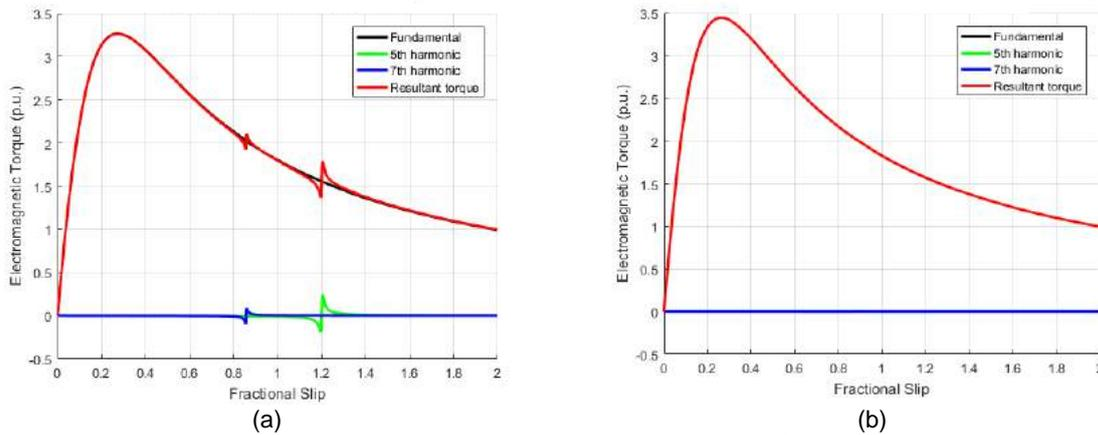
Fig. 31. Approximate motor electromagnetic torque curve considering the 5<sup>th</sup>- and 7<sup>th</sup>-order space harmonics of MMF: (a) original single-layer winding (Case 0); (b) optimized double-layer winding (Case 3).
