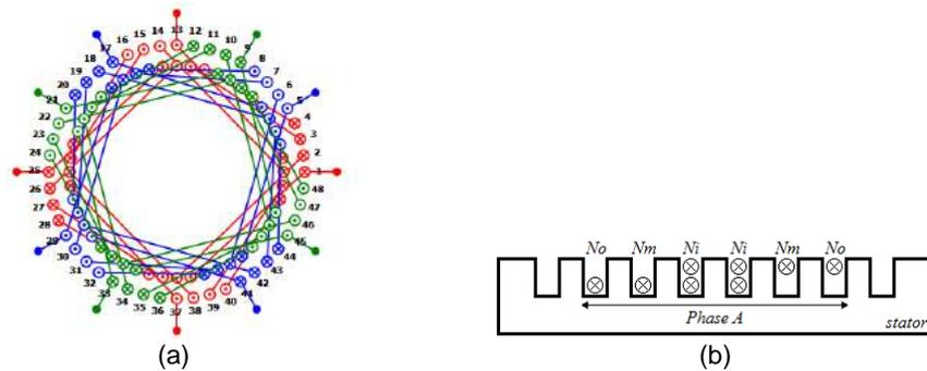
**Fig. 24.** Concentric, double-layer, 3-tier, stator winding configuration: (a) circular scheme; (b) identification of inner and outer coils.
