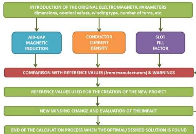
Fig. 13. Computing algorithm to improve or change the original winding design.
