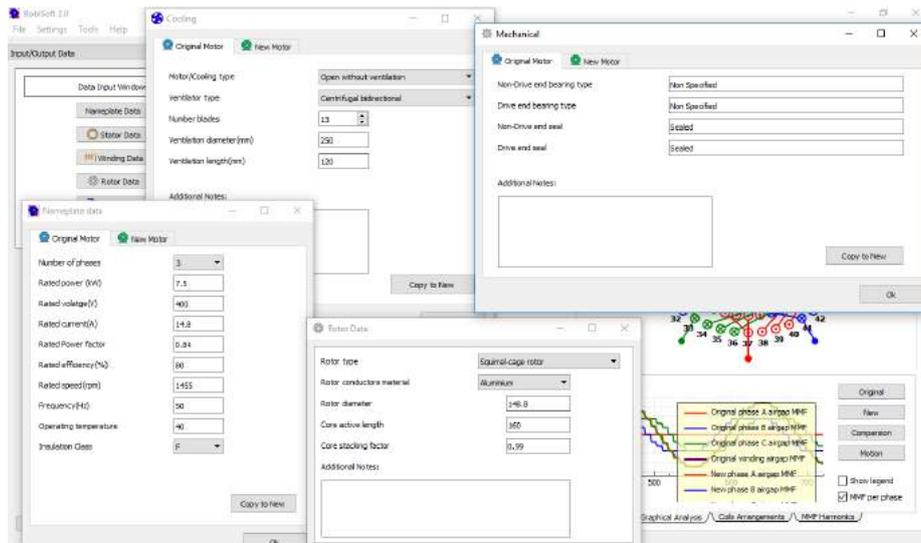
Fig. 15. Section to insert nameplate and mechanical data of the original and new motor.
