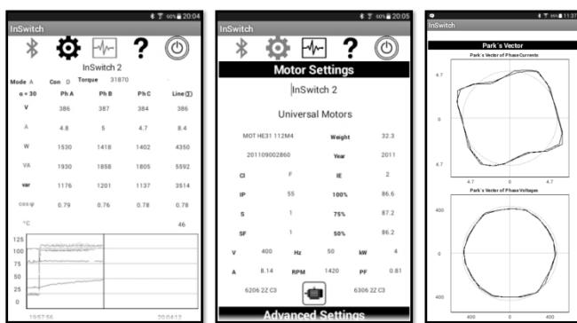
Allows configuring the InSwitch to a particular motor and displays the voltages, currents, active power, reactive power, power factor, electromagnetic torque and Park's Vector.
